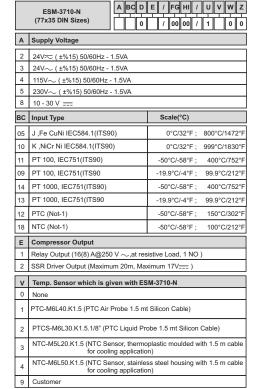
All order information of ESM-3710-N Temperature Controller are given on the table at above. User may form appropriate device configuration from information and codes that at the table at above. User may form appropriate device configuration from information and codes that at the table and convert it to the ordering codes.Firstly, supply voltage then other specifications must be determined. Please fill the
