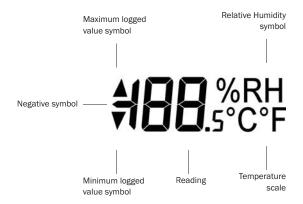
The LCD shows six different recorded readings, which can be cycled through using the built-in push button. The most recent logged value, maximum logged value and minimum logged value can be displayed separately for humidity and temperature. In addition, logging and alarm status is shown using two high intensity LEDs.
